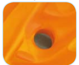
Enlarged front scupper holes for quick drainage
