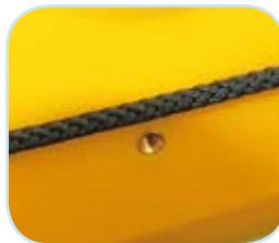
Mounting 'inserts' for insulated rear well cover and running rig
