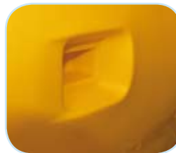
Recessed transducer scupper hole
